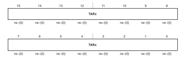
TARX Bits Timer\_A register. The TAR register is the count of Timer\_A. 15-0
